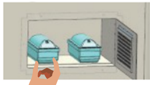
Twist and remove the filter
